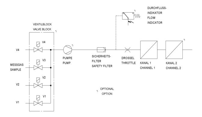
Fig. 1-3: Gas Flow Diagram: Single Channel or in Series
